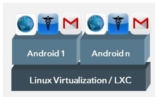
Figure 3: Full Android virtualization requires a separate instance per user, reducing user density.
