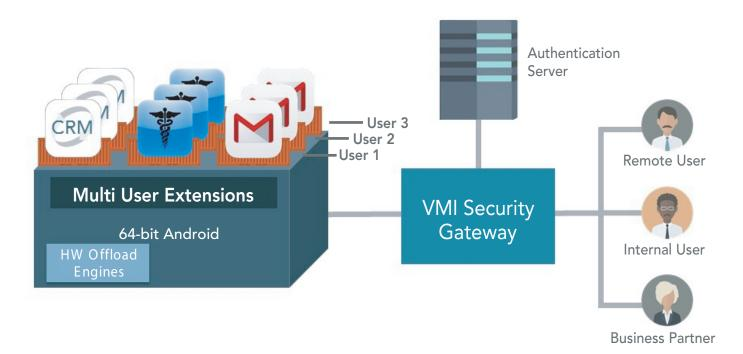
The SierraVMI architecture includes one or more multi-tenant Android virtual machines and a SierraVMI gateway that load balances connections to the Android virtual machines, performs management, and provides access to mobile apps.
